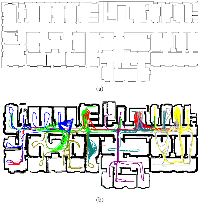
Fig. 8: a) Simulation environment. b) Trajectories and final map in a 8 robots experiment.
