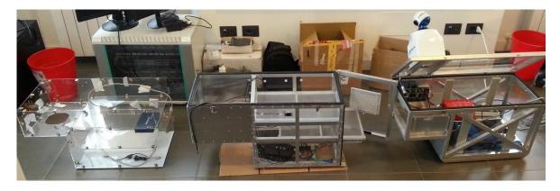
Figure 4 – Three iterations of the robot chassis design process.
