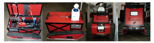
Figure 1 – The designed and constructed ROVINA robot (here depicted without the camera array).
