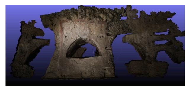
Figure 9 – High-resolution reconstruction of a portion of the catacomb obtained through SfM.
