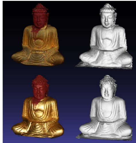
Figure 1. Top: s-o-a un-calibrated 3D reconstruction, with the shape rather smooth and Lambertian reflectance rendering. Bottom: proposed method with its refined geometry and extracted BRDF map.
